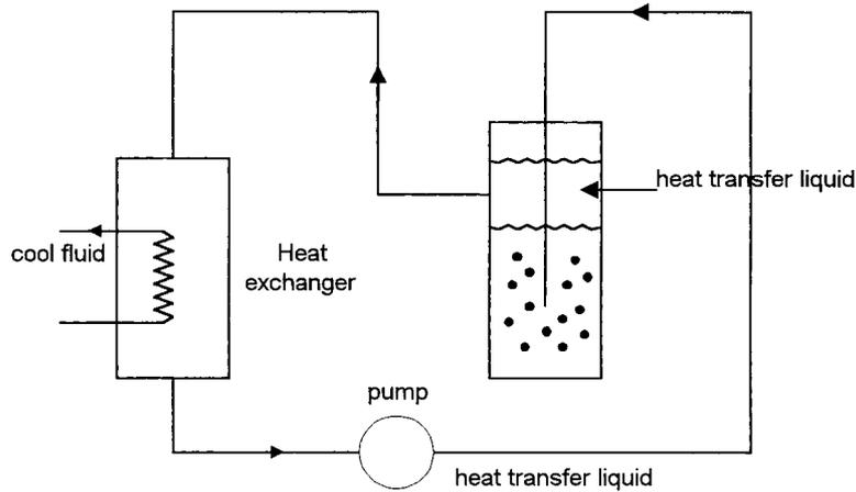
Fig. 1. Schematic of the direct-contact thermal energy storage.
