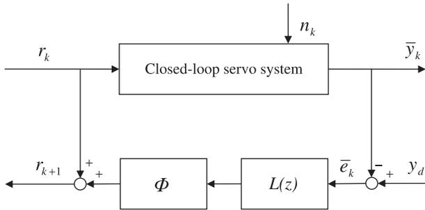
Fig. 2. Architecture of command-based ILC with measurement noise.
