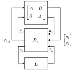
Fig. 4. Linear fractional representation of control problem.
