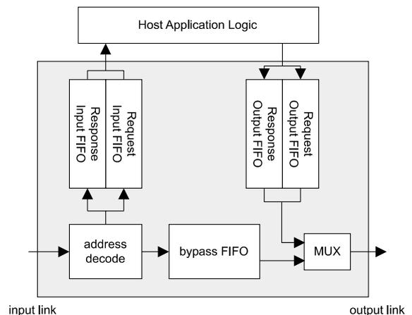
Fig. 1. High-level structure of an SCI node.
