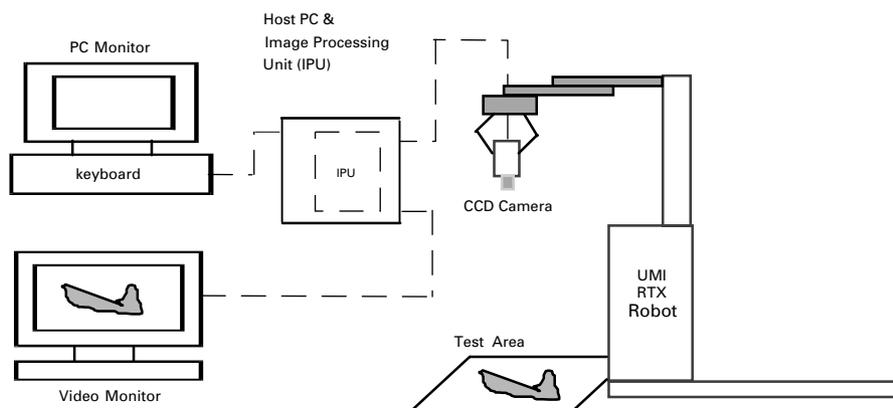
Fig. 2. Schematic representation of the test equipment.
