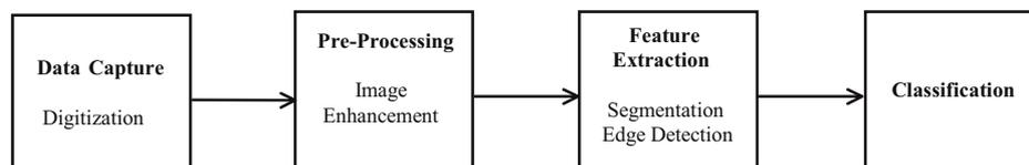
Fig. 1. Block diagram of a conventional visual pattern recognition system.
