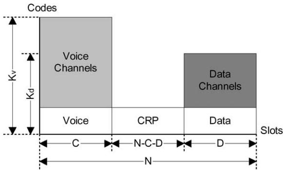
Fig. 1. DMBS frame structure.
