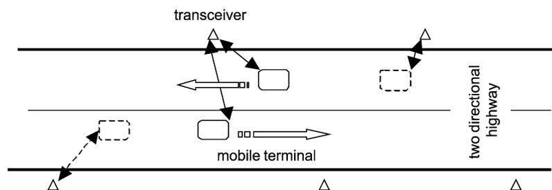
Fig. 2. Communication between mobile PC terminals and transceivers.
