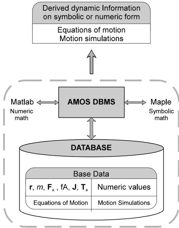
Fig. 1. The MECHAMOS system selects dynamic information derived from base data through a general QL.
