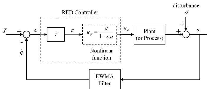
Fig. 2. A discrete-time representation of RED as pseudo-proportional controller.
