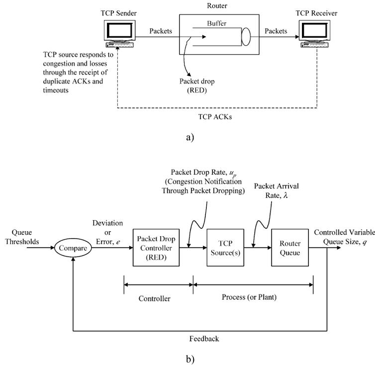
Fig. 1. (a) TCP congestion avoidance through random early detection, (b) TCP congestion avoidance as a closed-loop feedback control system.
