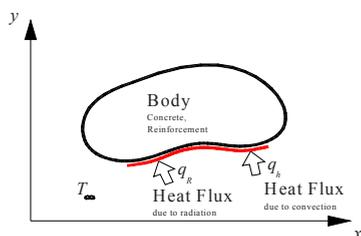
Fig. 1. 2-Dimensional conduction with surface convection (boundary condition).
