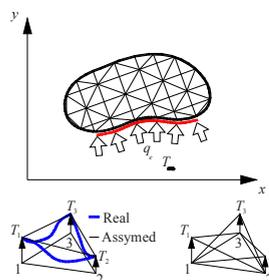
Fig. 2. Triangular element and real temperature vs. ideal temperature (shape function).
