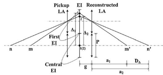
Fig. 3. Principle of the depth of reconstructed image.
