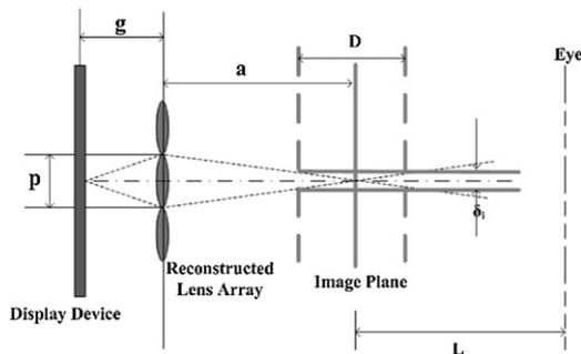
Fig. 2. 3DII system display parameters.
