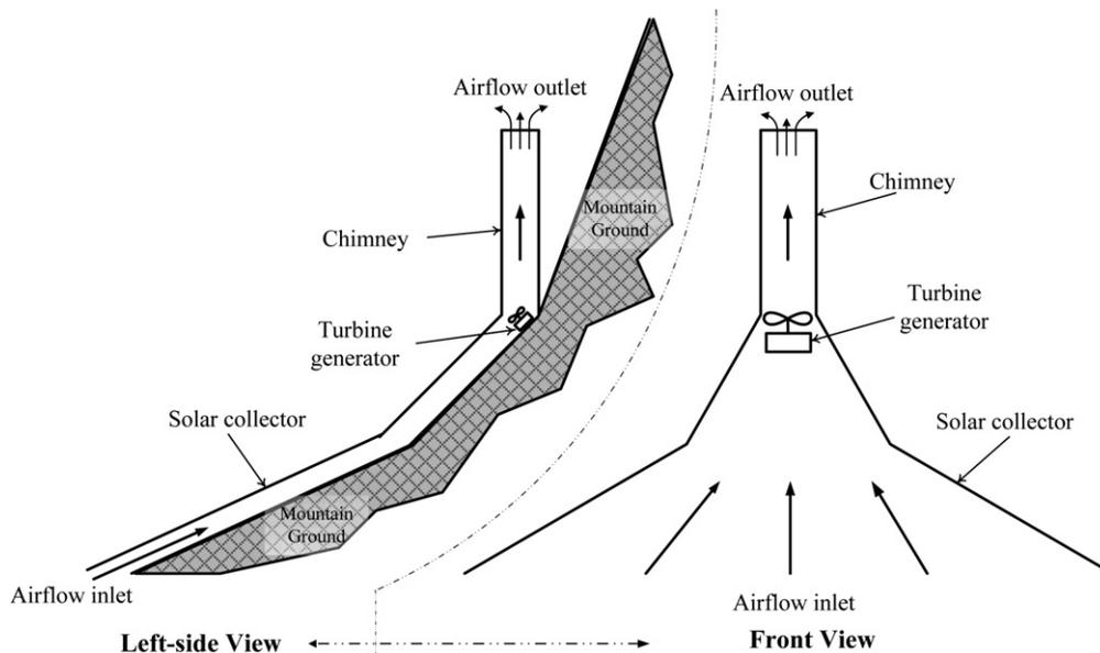
Fig. 2. Schematic of a sloped solar chimney power plant.
