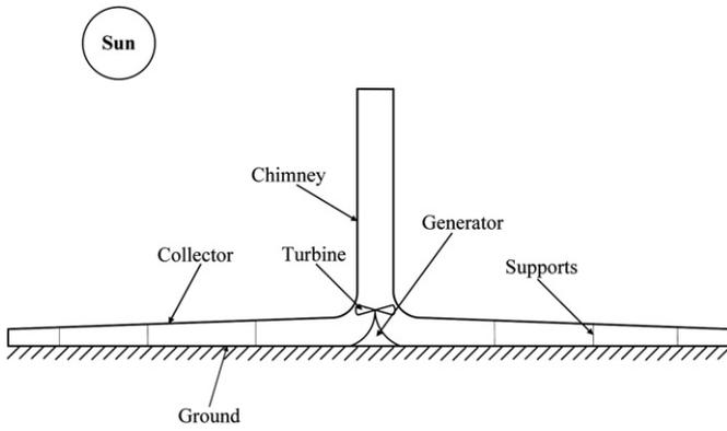
Fig. 1. Schematic of a solar chimney power plant.
