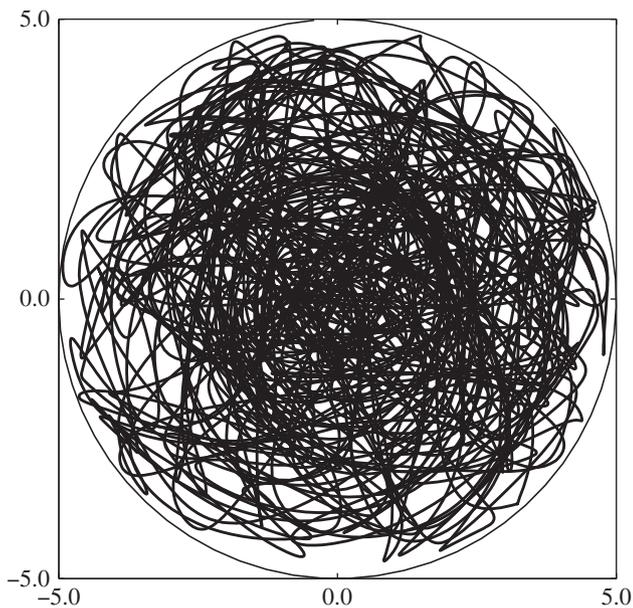
**Fig. 2.** Example of random track after 2 min of sliding. Track never crosses boundary circle of 10 mm diameter.
