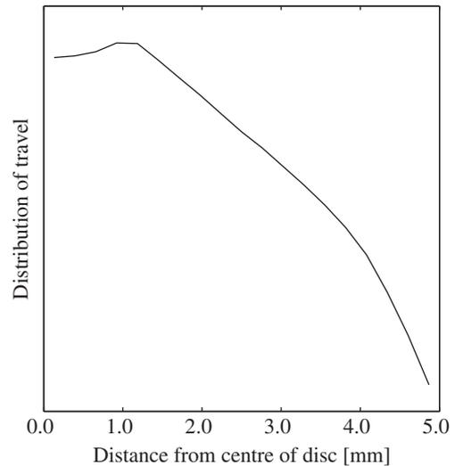
**Fig. 3.** Distribution of random travel on disc. A total of 360 000 points were computed, time interval being 0.01 s, corresponding to 60 min of sliding. In computation, disc was divided into 0.1 mm wide concentric rings, and total length of travel on each ring was divided by area of ring.
