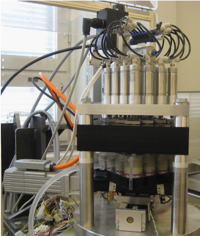
**Fig. 1.** RandomPOD wear test device with 16 test stations. Note servo-electric x-y-table for translation of discs, and proportional-pneumatic, vertical loading of pins. Test chambers are surrounded by circulating cooling water.
