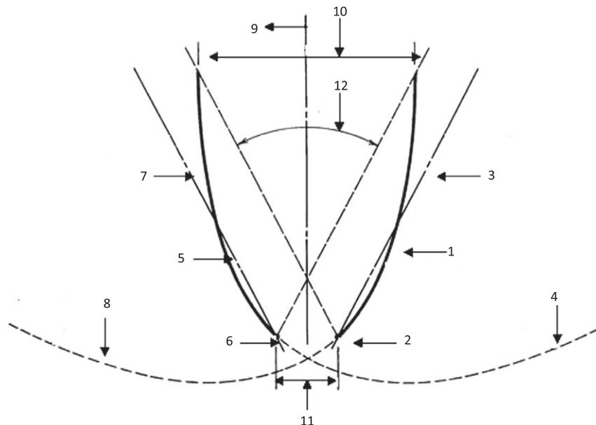
**Fig. 1.** The geometry of compound parabolic concentrator (CPC). (1) Parabola A, (2) focus of parabola A, ( $F_A$ ) (3) axis of parabola A, (4) truncated part of parabola A, (5) parabola B, (6) Focus of parabola B (FB), (7) axis of parabola (B), (8) truncated part of parabola B, (9) axis of CPC, (10) aperture of CPC ( $d_1$ ), (11) receiver opening ( $d_2$ ), (12) acceptance angle ( $2\theta$ ).
