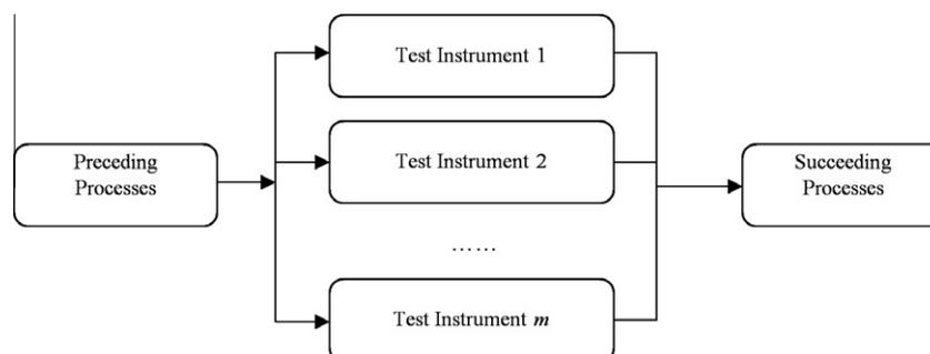
Fig. 1. A multisite testing system.
