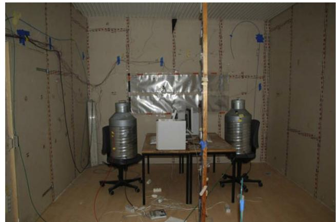
Fig. 1. Photo of the test climate chamber with an office layout.
