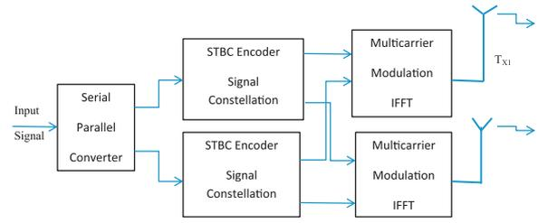
Fig. 1. System transmitter block diagram.
