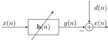
**Fig. 1.** Prototypical adaptive filter setup.
