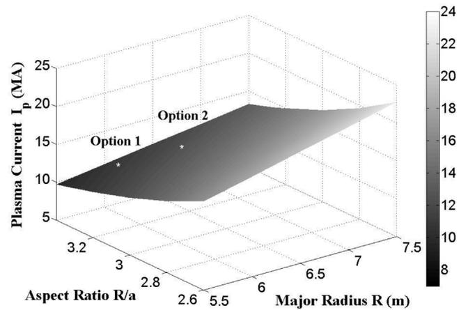
Fig. 2. Plasma current variation as a function of the aspect ratio and major radius when the toroidal magnetic field at the plasma core is 7.72 T.
