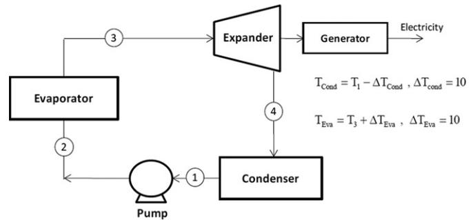
Fig. 1. Schematic of a typical Organic Rankine Cycle (ORC).
