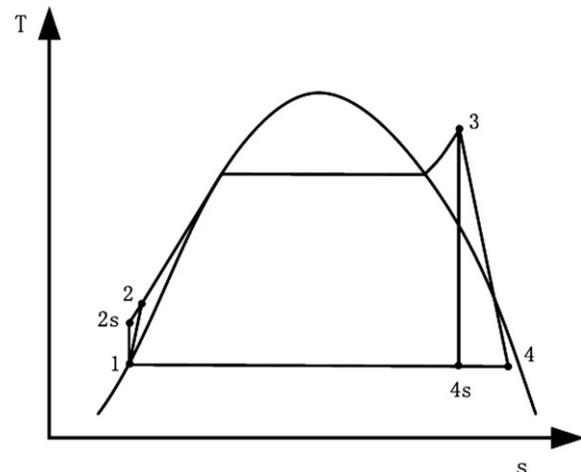
Fig. 2. ORC with a negative slope of the saturated vapour curve and wet vapour at the expander outlet.
