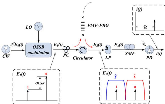
Fig. 1. Analytical model of the proposal with schematic spectrum (inserted); (CW, continuous-wave laser; LO, local oscillator; PC, polarization controller; PMF-FBG, polarization-maintaining fiber Bragg grating; LP, linear polarizer; SMF, single mode fiber; PD, photodiode).
