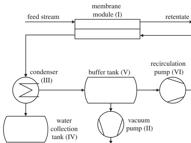
Fig. 1. Schematic representation of the membrane unit and the permeate side constituents of a humidity harvesting unit, working with water vapor selective membranes.
