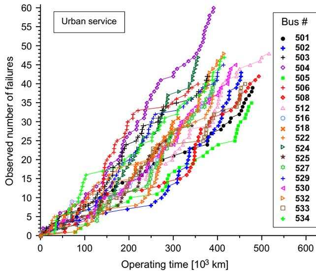
Fig. 1. The (interpolated) paths of the powertrain systems of buses employed in urban service.
