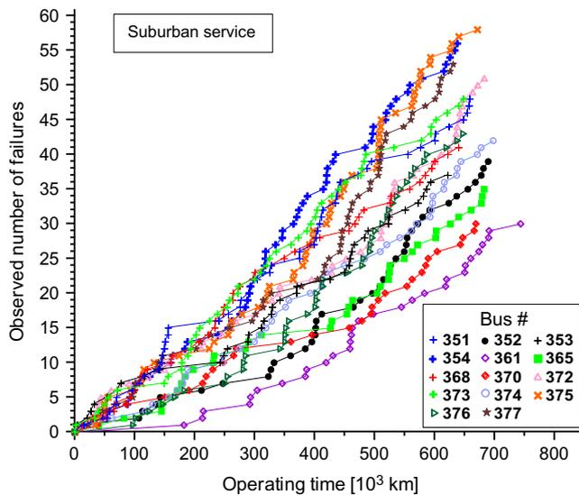
Fig. 2. The (interpolated) paths of the powertrain systems of buses employed in suburban service.
