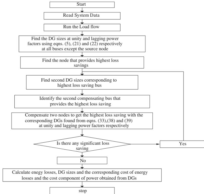
Fig. 1. Flow chart for DG allocation.
