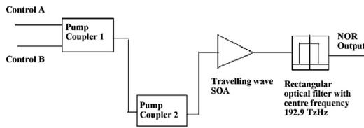
Fig. 1. The experimental setup for all optical NOR gate.
