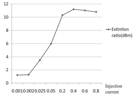
Fig. 3. Variation of extinction ratio with input injection current to SOA.
