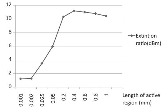
Fig. 4. Variation of extinction ratio with length of active region.
