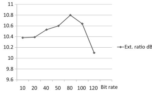
Fig. 2. Variation of extinction ratio with bit rate.
