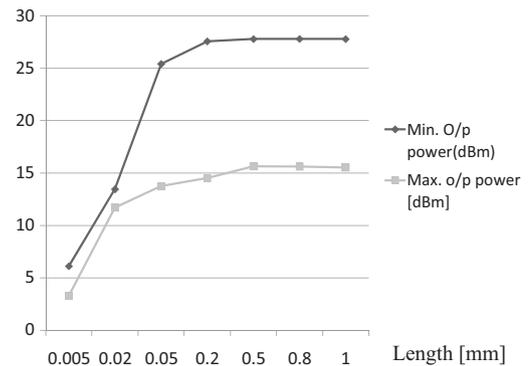
Fig. 5. Variation of minimum and maximum output (for level '1' and '0') with length of active region of SOA.
