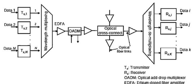
Fig. 1. Conceptual diagram for system's setup [William Shieh].
