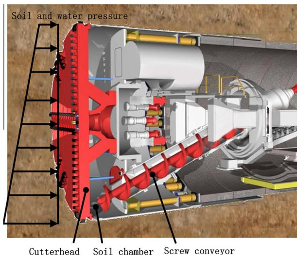
Fig. 1. Cutterhead system of EPB shield machine, modified from Herrenknecht website (<http://www.herrenknecht.com>).
