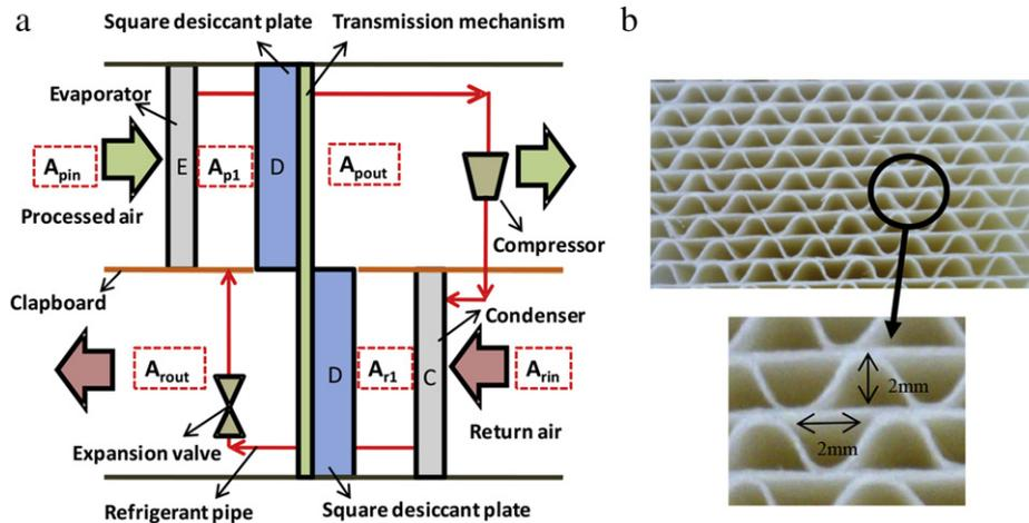
Fig. 1. Operating principle of the dehumidifier using solid desiccant: (a) single-stage dehumidifier; and (b) square desiccant plate material.
