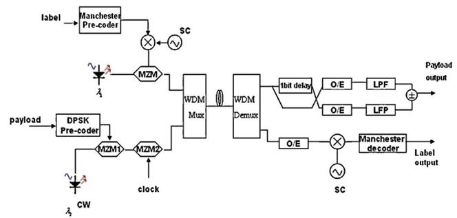
Fig. 3. Sending and receiving schematic of the second method.
