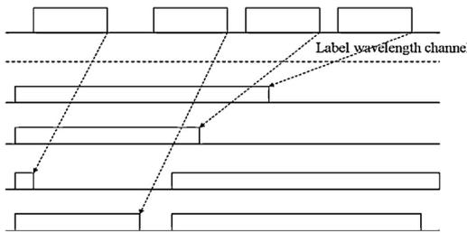
Fig. 1. Channels of dedicated wavelength optical label and multi-wavelength payload.
