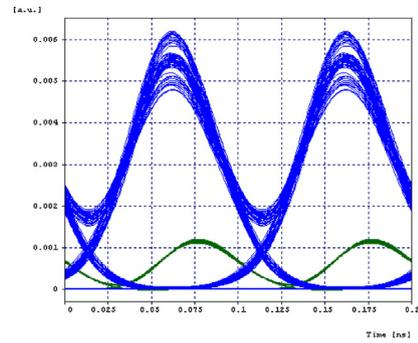
Fig. 3. Superimposed eye diagram of 4-channels.
