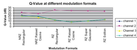
Fig. 5. Q-value at different modulation formats in 4-CATV transmission channels.
