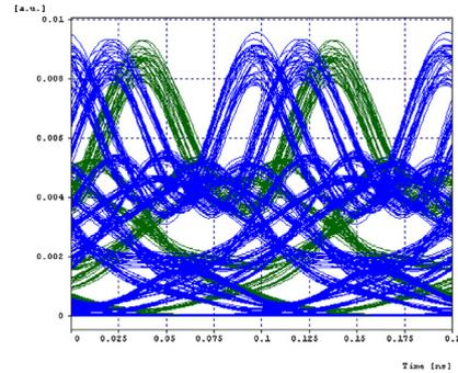
Fig. 4. Superimposed eye diagram of inserted and dropped channel 2.
