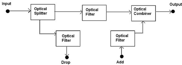
Fig. 1. Simple optical add-drop multiplexer [G.P. Agrawal].
