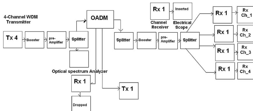
Fig. 2. Germanized block diagram for CATV 4-channel transmission system [Senior].
