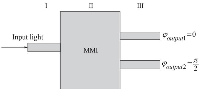
Fig. 1. Structure of  $1 \times 2$  MMI.
