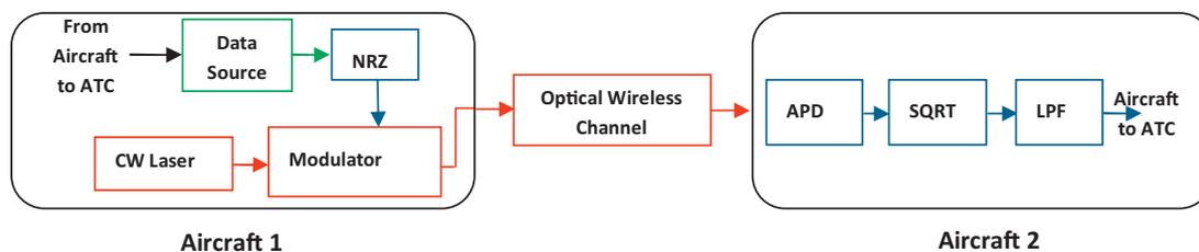
Fig. 1. Design of inter-aircraft optical-wireless communications systems.
