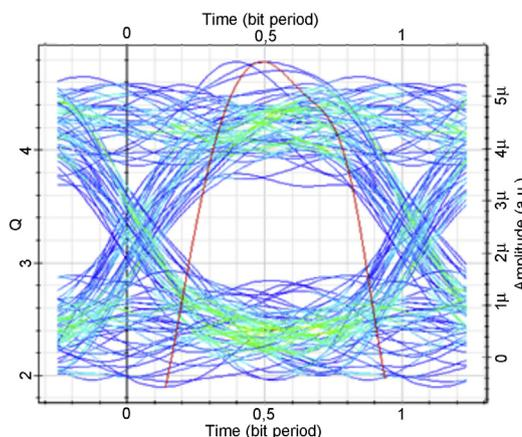
Fig. 3. Eye diagram of IaOWC system at 80 km.
