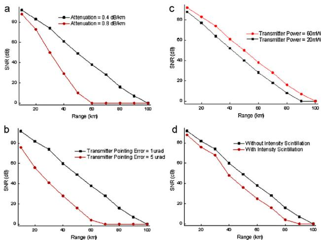
Fig. 2. (a) Evaluation of SNR (dB) versus range with different attenuation. (b) Evaluation of SNR (dB) versus range with different transmitter pointing error. (c) Evaluation of SNR (dB) versus range with different transmitter power. (d) Evaluation of SNR (dB) versus range with an without Intensity Scintillation.
