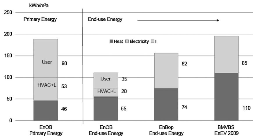
**Fig. 1.** Energy consumption for 12 selected EnOB office buildings (end-use energy and primary energy) compared to data from consumption-based energy certificates according to the actual German Energy Conservation Regulation EnEV 2009 [4] and from a cross-sectional analysis of 30 recently built modern office buildings according to an evaluation within EnBop. User related electricity consumption includes IT and all other appliances for office work.
