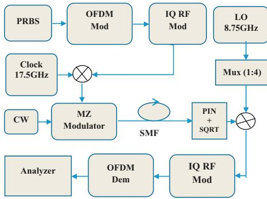
Fig. 1. Simulation setup of a high speed OFDM-RoF transmission links.
