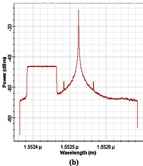
Fig. 2. Electrical and optical spectrum of (a) OFDM-RF mixed signal and (b) OFDM-RoF using SSB modulation scheme.
