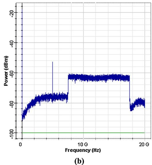
Fig. 3. Electrical spectrum of OFDM-RoF transmission links with (a) OSSB modulated data after optical span of 0 km and (b) OSSB modulated data after optical span of 50 km.
