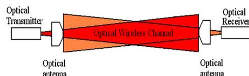
**Fig. 2.** Optical antenna increase the signal divergence.
