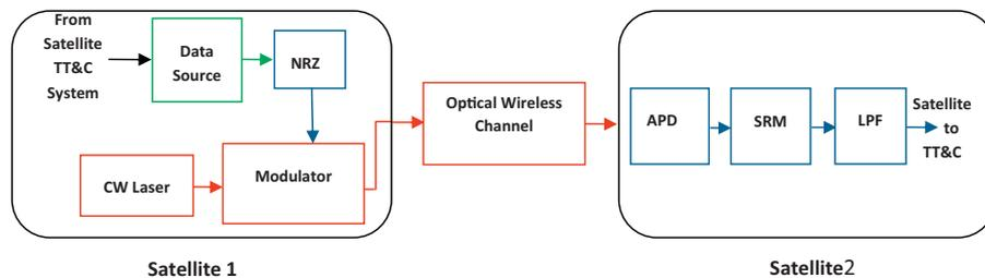
**Fig. 1.** Basic block diagram of an inter-satellite optical-wireless communications system: CW Laser; LPF, low pass filter; APD, Avalanche Photo detector; TT&C, Telemetry, Tracking and Communication systems.
