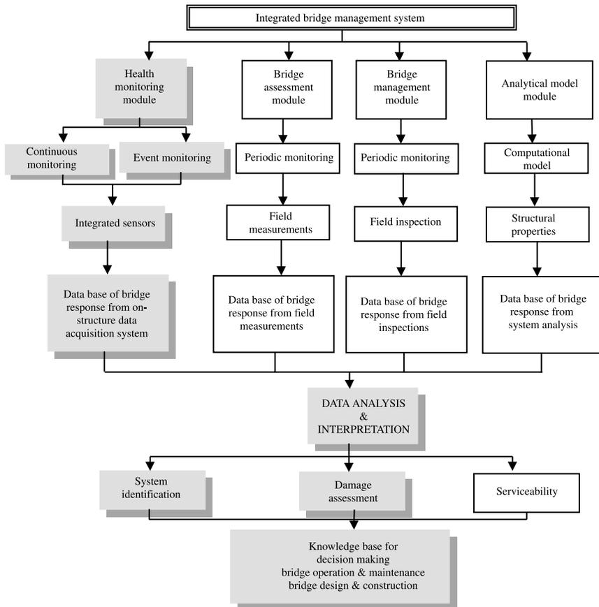
Figure 1. An integrated bridge management system.
