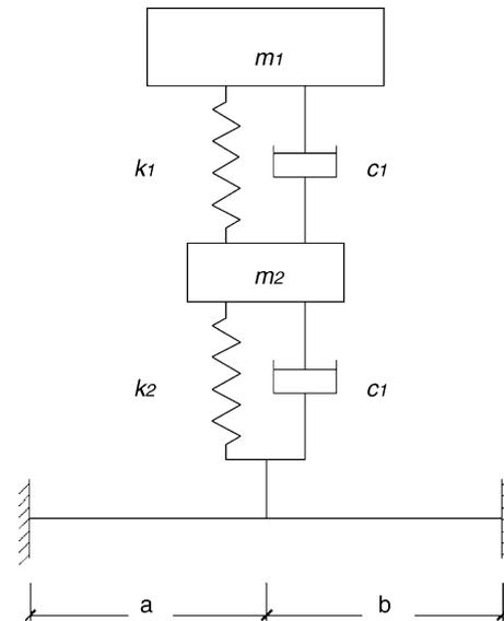
Fig. 1. A quarter car model attached to a beam at an arbitrary point.
