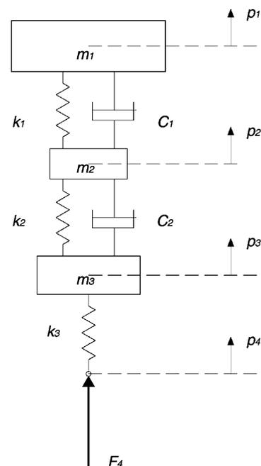
Fig. 2. Mathematical model of car-beam system.
