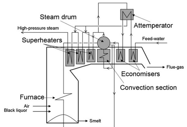
Fig. 1. Recovery boiler.
