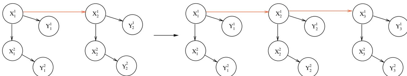
Fig. 1. Because of parameter tying, a DBN can be represented by only two time slices (left). To fit the two observation sequences  $\{Y^1\}$  and  $\{Y^2\}$  of length  $T = 3$ , the DBN is unrolled and represented on 3 time slices (right).
