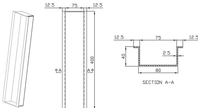
Fig. 1. Generic profile geometry of cast AM60 component without ribs.
