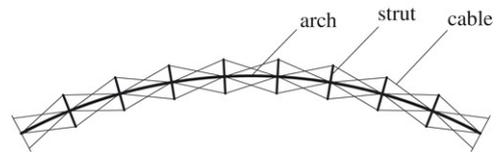
Fig. 1. A cable-stiffened arch.
