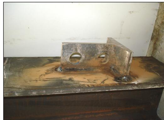
Fig. 2. T-Perfobond shear connector.
