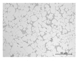
**Fig. 1.** Typical microstructure of an HPDC AlSi4Mg alloy. The primary  $\alpha$ -Al crystals appear with light grey tone, while the Al–Si eutectic appears darker. Some Fe-, Mn-bearing intermetallic particles are present with approximately similar grey-tone as the eutectic.
