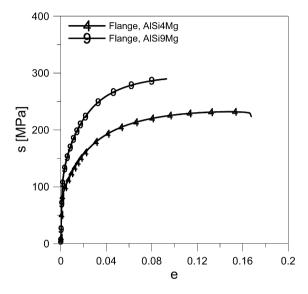
**Fig. 4.** Typical engineering stress-strain curves obtained from uniaxial tensile tests of AlSi4Mg and AlSi9Mg.
