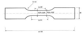
Fig. 3. Geometry of tension test specimen [mm]. Picture is scaled from original.
