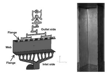
**Fig. 2.** Left: Illustration of the generic HPDC U-profile with length of 300 mm and thickness of about 2.5 mm and corresponding gating system. Right: Picture of casting in axial crushing rig.
