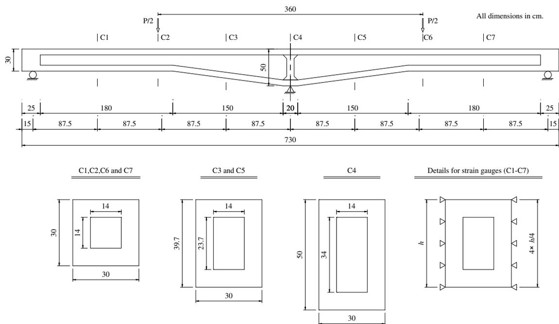
Fig. 1. Geometrical configuration of the test beam.
