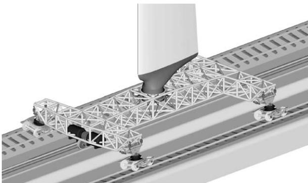
Fig. 2. Structural configuration of a blade-wagon showing the bogies, the suspension system and the electrical generators coupled to their driving wheels.
