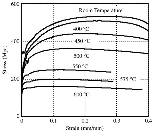
Fig. 2. Stress–strain relationship of steel at elevated temperature.
