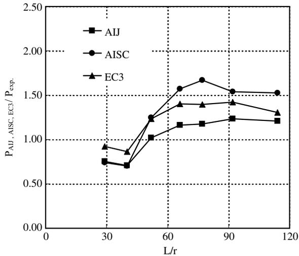
Fig. 1. Comparisons of A36 steel column strength at 500 °C.
