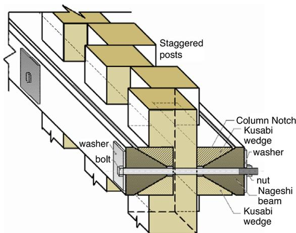
Fig. 2. K-N joint shear wall with staggered columns.
