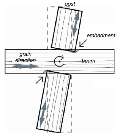
Fig. 3. Embedment and grain direction.
