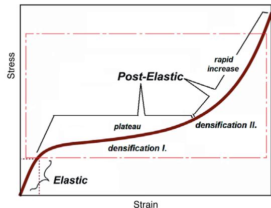
Fig. 4. Partial compression stress–strain curve.
