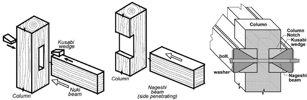
Fig. 1. Traditional Nuki joint (left), Nageshi (centre) and the new K-N joint (right).
