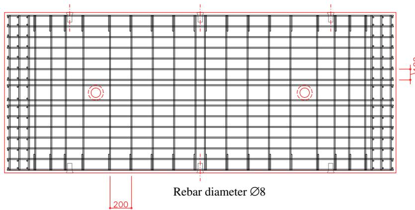
Fig. 2. Tunnel segment reinforcement.
