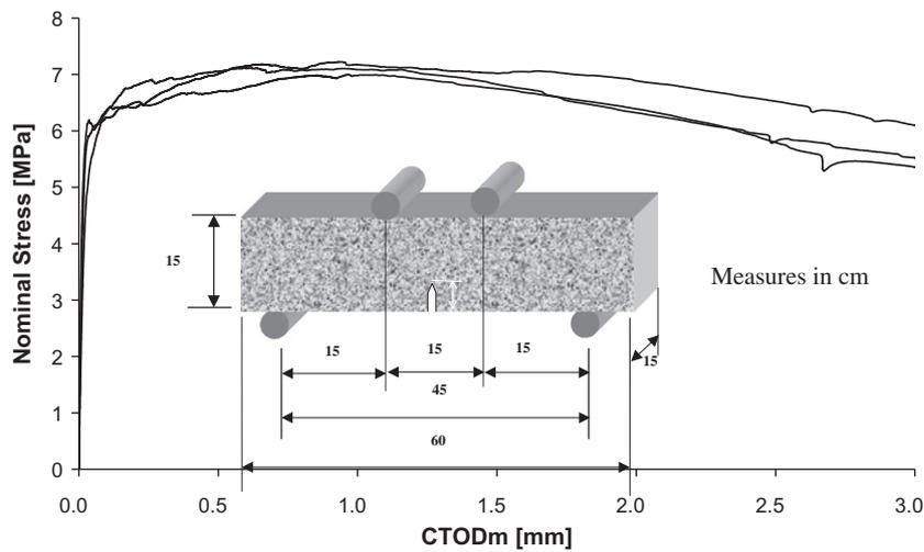
Fig. 3. FRC flexural behaviour in tension: nominal strength versus crack opening.
