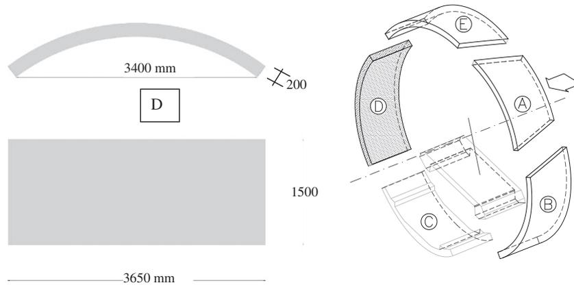
Fig. 1. Tunnel segment geometry.
