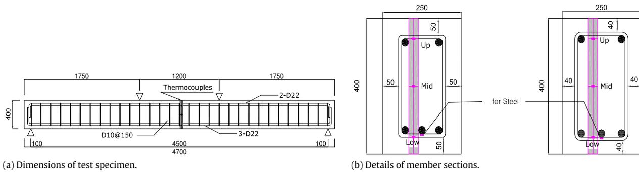
Fig. 1. Configuration of fire test beam and location of thermocouples in the sections (unit: mm).
