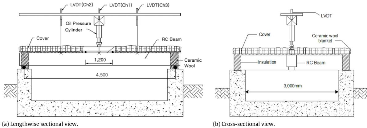
Fig. 2. Test set-up of a beam in the fire chamber (unit: mm).
