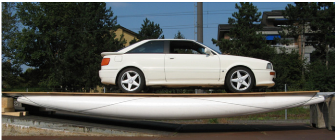
Fig. 1. Test under operational conditions of the Tensairity demonstration bridge with 8 m span.
