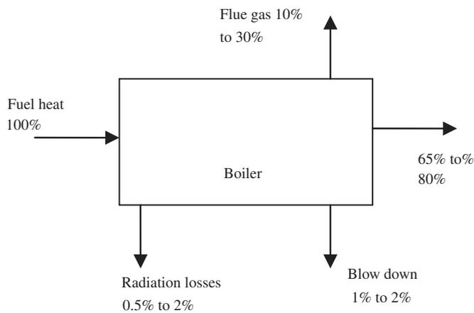
Fig. 1. Typical heat balance of a boiler (Jayamaha, 2008).
